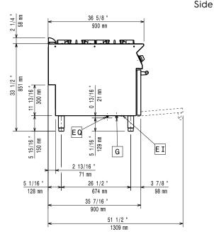
Electrical inlet (power) Gas connection
