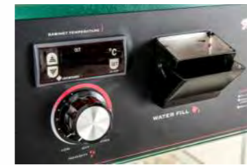
1. Thermostat control(30-85°C) with manual water refill inlet
