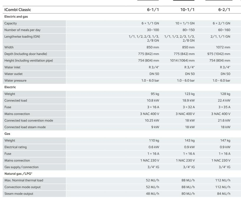
\* To guarantee proper operation, the appropriate connection flow pressure must be ensured: Natural gas H G20: 18-25 mbar mbar (0.261-0.363 psi), LPG G30 and G31: 25-57.5 mbar (0.363-0.834 psi). ENERGY STAR available for cooking systems 6-1/1 and 6-2/1 in electric and gas as well as 10-1/1 electric. iCombi Pro (LM100) and iCombi Classic (LM200) models are NSF certified as can be seen on the NSF listing
